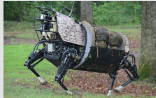
DARPA is sponsoring development of an advanced version of the Legged Squad Support System (LS3) robot, shown above.
