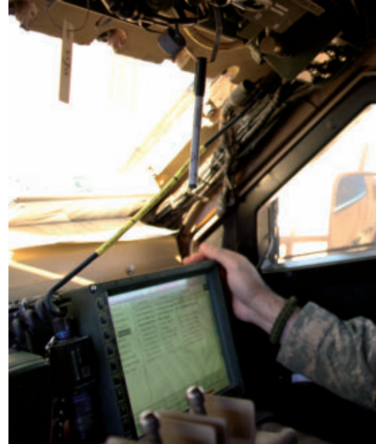
The Mounted Family of Computer Systems (MFoCS) program will build rugged computers for land vehicles, which subject data storage to massive amounts of shock and vibration.
